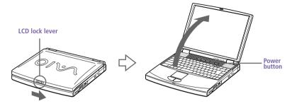
Press the power button on top of the computer until the green power indicator light turns on.
